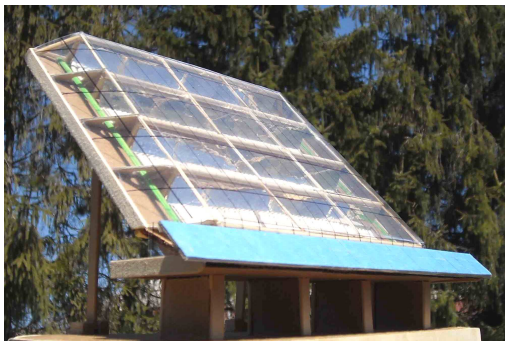
Fig. - BI-ET&R test facility components: a) Solar Collector (evacuated tubes, etc.); b) Interior Reflectors; c) Exterior Glazing Aperture (EGA)
